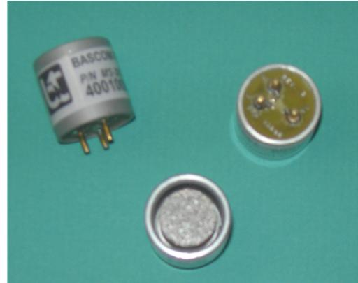
Bascom-Turner methane sensors are not significantly affected by chlorides or sulfides because of their composition and operating temperature. Airborne lead concentrations have been reduced essentially to zero ever since lead compounds were removed from gasoline. What remains as a potential poison is silicon derived from commercial silicones with an appreciable vapor pressure.
