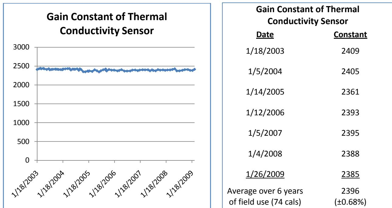
Box 1. Gain constant for typical thermal conductivity sensor tracked over 74 calibrations and 6 years of field use (graphical and tabular views show same data.)
