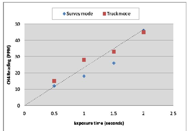
Figure 4. Instrument response to short (0.5 to 2 second) samples of 50ppm methane.
