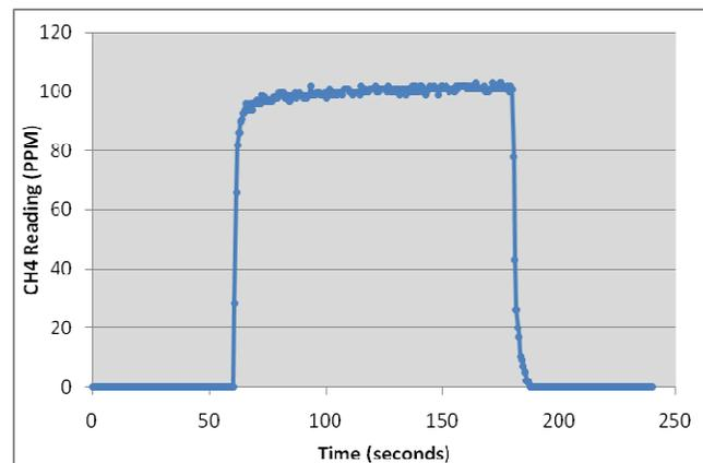
Figure 3. Instrument response to sustained sample of 100ppm methane.
