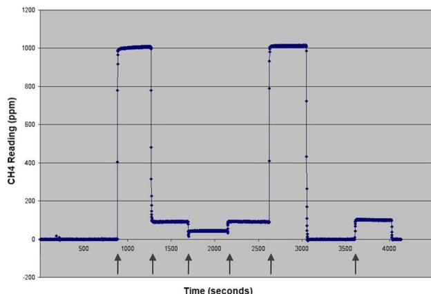
Figure 2. Instrument response to 50ppm, 100ppm and 1000ppm methane, given in random order.
